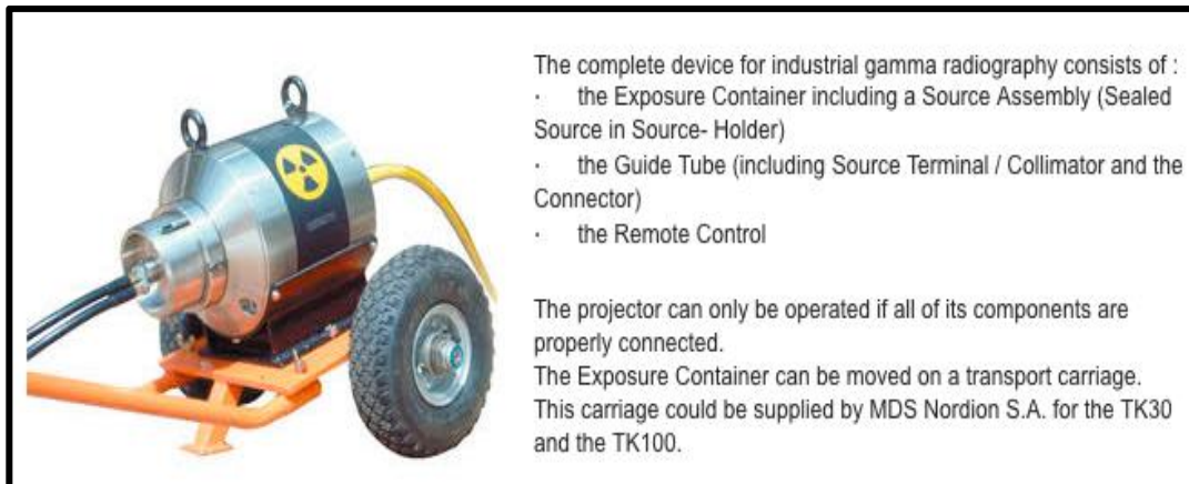
Industrial gamma radiography device on towed carriage. Source Projector: TK-100
